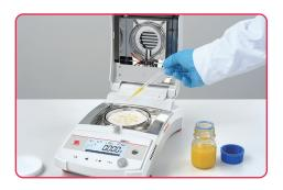
An LCD with second line display, navigation knob, and intuitive operation makes for convenient and easy routine moisture testing.
