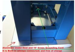
BenchPro provides built-in left and right wrist strap Jack and 10' grounding cord installed on frame.
