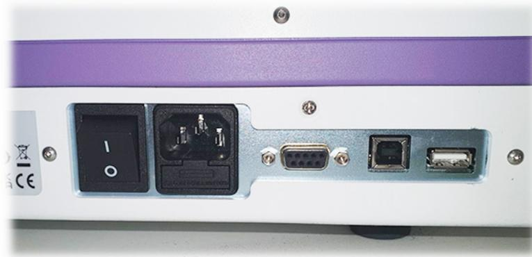
**Figure 5-2: RS232 and USB Ports on an Automated Individual Access Roll Heat Sealer**
