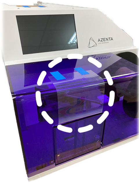
A photograph of the Azenta Life Sciences device. The device is white and purple. A dashed white circle is drawn around the seal roll area, indicating where to peel off the pull end of the leading seal.                                                 |
