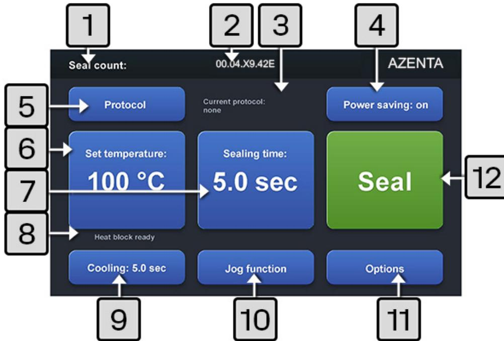
Figure 2-3: Automated Individual Access Roll Heat Sealer Screen Features
