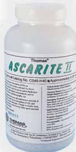
Ascarite II is the universally-accepted carbon dioxide absorbent. It captures and contains CO<sub>2</sub> through chemical change making it a non-regenerative consumable product.
