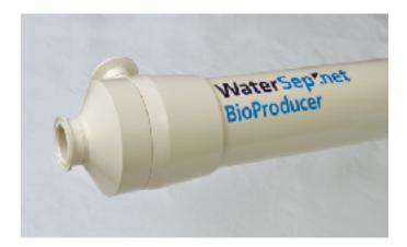
The BioProducer24 ReUse is a production scale hollow fiber cartridge designed for biopharmaceutical concentration/diafiltration and clarification unit operations. With a surface area of 2.7 m<sup>2</sup>, the BioProducer41 ReUse HF cartridge can accommodate batch volumes between 50 L and 280 L with a typical process flow of 135 L/hr.
