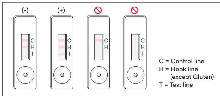
Any reading after 12 minutes from the initial application of the sample into the 3M Fish Protein LFD should be considered invalid. A reading at this time cannot be interpreted and can lead to erroneous results.
