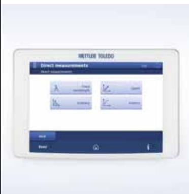
Spectrum scans, fixed wavelength absorption measurements, quantification with calibration curves or kinetic analyses are ready to use as direct measurements: Simply enter parameters, define the preferred workflow, store as a shortcut, and start the measurement with One Click.
