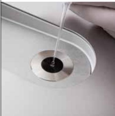
Micro-volume UV/VIS measurement is the method of choice when measuring either small sample amounts or high absorption samples. Only 1  $\mu\text{L}$  of sample is required for reliable measurements. The pure sample is pipetted on the measuring surface and the arm is locked automatically to a precisely defined pathlength. Measurement errors are avoided, as the sample does not need to be diluted.
