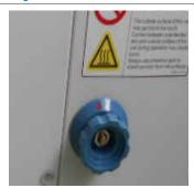
Three way Drain Valve Handle
