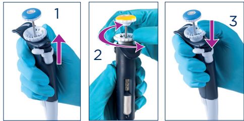
Figure 5 Volume unlock and lock
