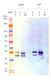
Western blots were detected under reduced conditions with anti-EBOV VP40 mAb 3G5 at 10 ng/mL and visualized using an anti-mouse IgG-HRP conjugate and TMB membrane substrate. rVP40 was loaded at 100 ng per lane. SUDV rVP40 and EBOV rVP40 are visualized in lanes 1 and 2, respectively. VLP was loaded at 1  $\mu g$  per lane. VP40 is detected in SUDV VLP (lane 4) and EBOV VLP (lane 5).
