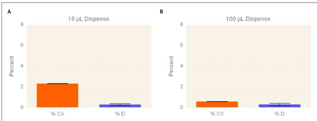
**Figure 1. Analysis of EV-100-R tip with aqueous dispense.** The precision (assessed by % CV) and accuracy (assessed by % D) of Axygen EV-100-R tips dispensing (A) 10 µL and (B) 100 µL volumes using the MCA head on the Tecan Freedom EVO liquid handling workstation were determined using the Artel MVS® system. The % CV and % D were below 2.5% for 10 µL and below 1.0% for 100 µL dispenses, n = 288.
