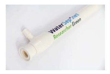
The Researcher Green crossflow hollow fiber membrane cartridges are designed for pilot scale and small scale production. It is the perfect tool for process development. With a surface area of 1,720 cm², the Researcher41 Green can accommodate batch volumes that range from 1,000 ml to 8,000 ml with a typical permeate flow rate of 5.2-10 L/hr for ultrafiltration applications and 3.4-6.9 L/hr for microfiltration applications.
