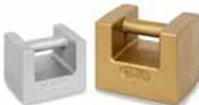
Cast Iron Grip Handle Weights are manufactured in sizes ranging from 2 kg through 2000 kg and 5 lb through 5000 lb. Weights are available in ANSI/ASTM E617 Class 4, 5, 6, 7 and NIST Class F. (2 kg and 5 lb weights are not available in Class F)
