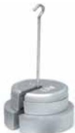
Cast Iron Slotted Weights are manufactured in sizes ranging from 200 g through 100 kg and ½ lb through 200 lb. Weights are available in ANSI/ASTM E617 Class 4, 5, 6, 7.
