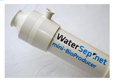
The mini-BioProducer24 ReUse series of cross flow hollow fiber membrane cartridges are designed for pilot scale and medium scale production and is the perfect tool for process development. With a surface area of 1.35 m², the mini-BioProducer24 ReUse can accommodate batch volumes that range from 25L to 140L with a typical process flow of 67.5L/hr.
