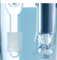
Due to the standard addition technique procedure, no calibration is necessary. Just carry out the automated Sensor conditioning and immediately start the analysis.
