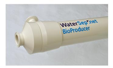
The BioProducer41 ReUse is a production scale hollow fiber cartridge designed for biopharmaceutical concentration/diafiltration and clarification unit operations. With a surface area of 5.0 m<sup>2</sup>, the BioProducer41 ReUse HF cartridge can accommodate batch volumes between 75 L and 500 L with a typical process flow of 250 L/hr.
