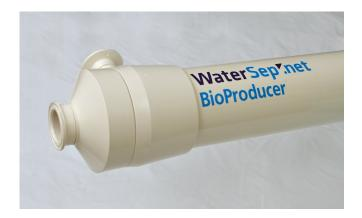
The BioProducer12 ReUse is a production scale hollow fiber cartridge designed for biopharmaceutical concentration/diafiltration and clarification unit operations. With a surface area of 1.2 m², the BioProducer12 ReUse HF cartridge can accommodate batch volumes between 25 L and 100 L with a typical process flow of 60 L/hr.
