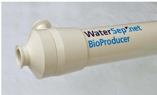
The **BioProducer12 ReUse** is a production scale hollow fiber cartridge designed for biopharmaceutical concentration/diafiltration and clarification unit operations. With a surface area of 1.2 m<sup>2</sup>, the **BioProducer12 ReUse HF** cartridge can accommodate batch volumes between 25 L and 100 L with a typical process flow of 60 L/hr.
